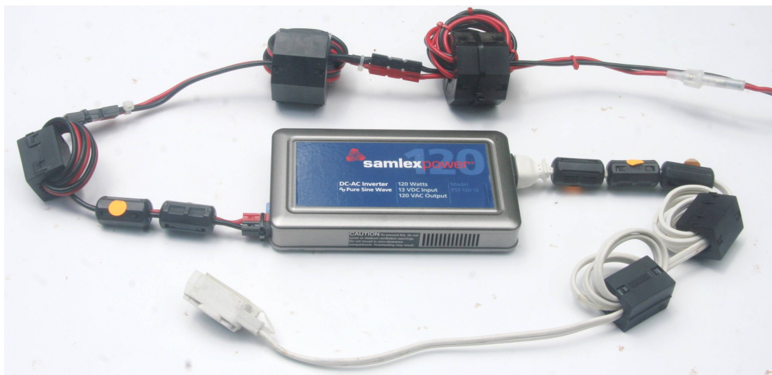
Fig 11 – 12VDC to 120VAC 1A Inverter with Required RF Filtering
