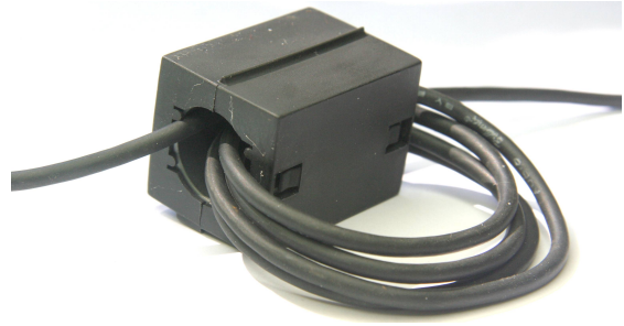
Fig 7 – 5 turn choke, good for 7-30 MHz
